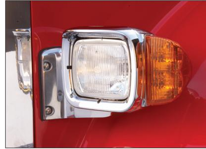
New pod-mounted headlamps are durable and corrosion-resistant, and feature halogen complex reflector technology for 50% greater low beam performance and nearly 600% longer bulb life.
