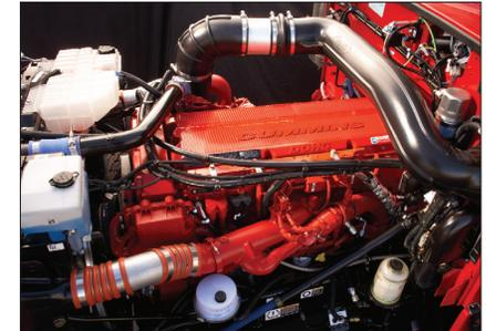
A new lightweight, high-capacity cooling module increases cooling efficiency for high horsepower applications and features a new fan ring shroud design for improved underhood airflow.
