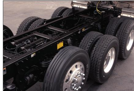
The Model 367 can be spec'd with a variety of heavy duty components including full and partial frame liners, as well as a selection of axles including tandem, tridem and lift-axle options.
