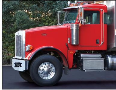
The gently sloped, long-length hood on the Model 367 not only enhances visibility, it allows for a 1,438 square-inch radiator to accommodate engines of up to 600 HP.
