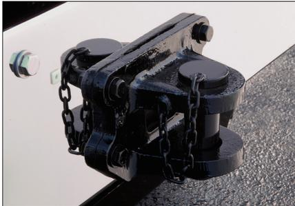
Bumpers on the Model 367 accommodate both a center tow hook configuration and a dual removable pin configuration that meet TMC towing guidelines of 80,000 pounds.
