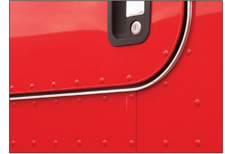
A lightweight, huckbolted, all-aluminum cab with lap seam construction and bulkhead style doors is legendary for toughness and corrosion resistance. It provides years of virtually water-tight performance.
