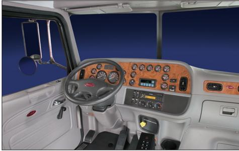
The rugged ProBilt interior features contoured door panels, an ergonomic dash with burl woodgrain, LED backlit gauges, five grab handles, a powerful HVAC system and durable, easy-to-clean materials.
