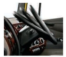
The steering wheel is generously adjustable: 8.5 cm in reach and between 30° and 45° in angle.
