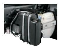
The compact lay out of the DAF SCR installation leaves enough free space on the chassis for large fuel tanks and other equipment.
